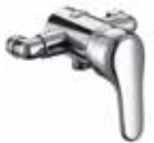
Alpha Valve Only - 15mm Manual valve suitable for exposed or concealed installation - Adjustable centres 130-160mm
